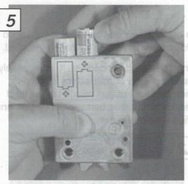
Your Pulsetronic lock requires two 3-volt lithium batteries. We recommend Duracell or Panasonic # CR123A cells. Always install NEW, unused batteries.
