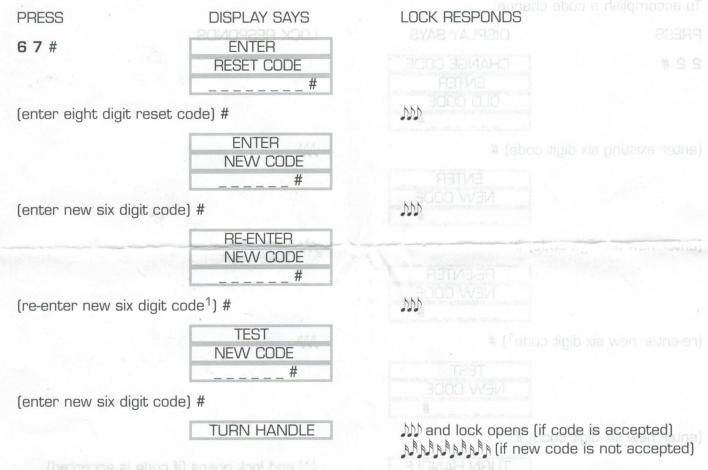
Enter your new code, followed by # to verify that it opens the lock. Open the safe door, and check the new code at least three times before closing the safe door.
