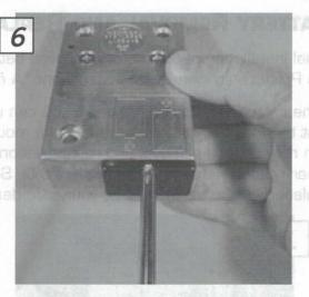
Install the battery cover, and secure it with the single screw you removed earlier. Do not overtighten.
