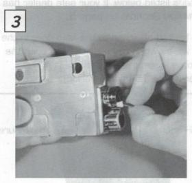
Remove the battery compartment cover. Note that it has a tab that mates with a depression in the bottom of the battery compartment.
