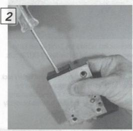
Remove the battery compartment cover screw. If there is enough room, battery replacement can be done with the lock still mounted to the safe door. The lock shown here has been removed from the safe for battery installation.
